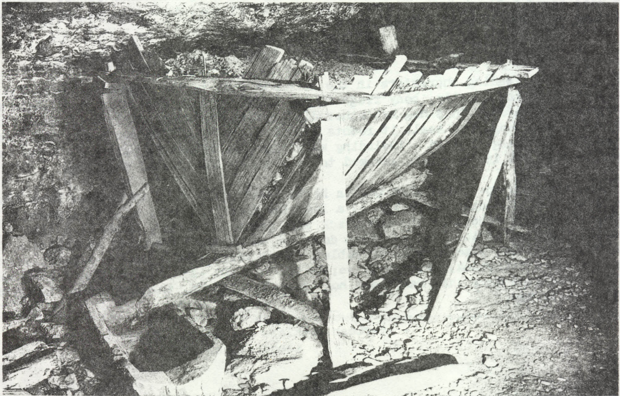
View of one of the 37 wood hoppers used in making gunpowder in Organ Cave.
